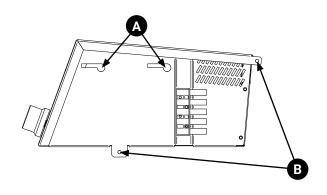
I) Loosen the screws (point **B**) from the smoker housing. Mount the electronic panel so that the holes in the panel align with the screws (point **A**). Slide the panel toward the back wall of the smoker until the connectors on the panel and smoker connect. Insert and tighten the screws in the correct locations (point **B**).
