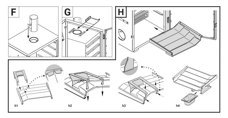
H) Install the drip tray holder before inserting the drip tray. To do so, turn the tray over and insert the hooks as shown in figure h1). Then attach the handle onto the edge of the tray as shown in figure h2) and h3). Turn the tray back over, place it in the smoker and insert the tray as shown in figure h4).
