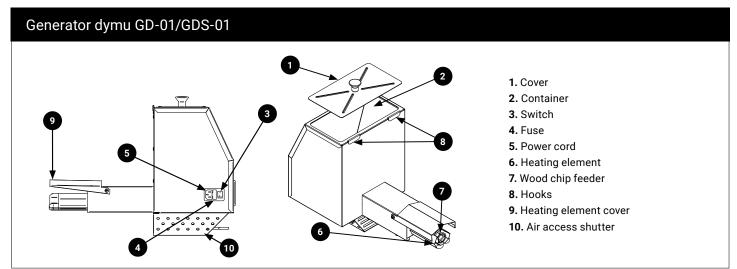
► After the smoke generator is started, the wood chip feeder (7) starts to rotate and the heating element (6) starts to heat up. The feeder continuously transports the chips from the container (2) to the surface of the heating element.
