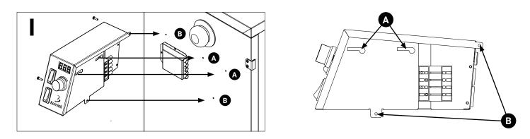
I) Loosen the screws (point **B**) from the smoker housing. Mount the electronic panel so that the holes in the panel align with the screws (point **A**). Slide the panel toward the back wall of the smoker until the connectors on the panel and smoker connect. Insert and tighten the screws in the correct locations (point **B**).
