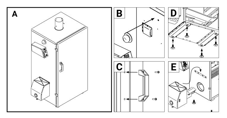
A) Remove the device from the box, discard any unnecessary packaging and read the user manual. B) Attach the carrying handles. C) Attach the door handle. D) Set the device in the appropriate location, tilt it slightly, screw the feet into the sockets on the bottom and adjust them to ensure that the device is level and upright. E) Insert the smoke generator heating element into the hole on the left wall. Tilt the generator slightly to attach it to the hooks.
